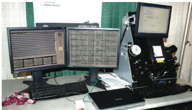
Equipment for digitizing microfilm features dual-screen display and mechanisms for orienting and enhancing digital images for online use.
